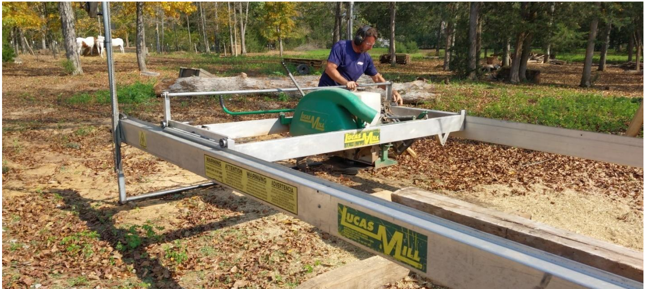
Timbers being sawed into siding
